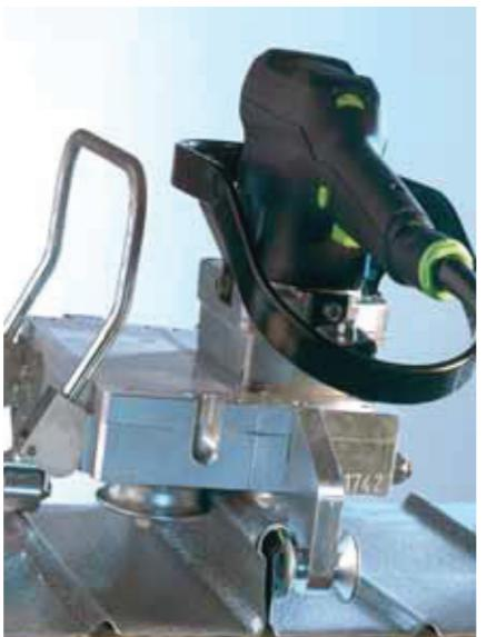
The mechanical zipping of the seams produces a load bearing connection. Vapor diffusion, however, is still possible in this area enabling residual moisture to evaporate after the installation.
